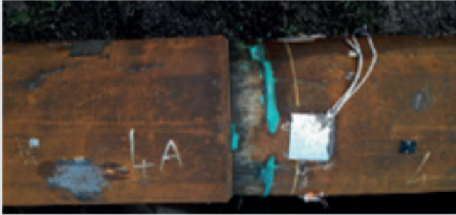
Figure 16: Compression to Failure
