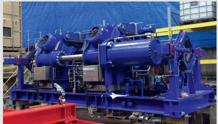
Figure 2: 10-16 inch - Zap-lok Press for up to 1.000" wt and grade X65 pipe
