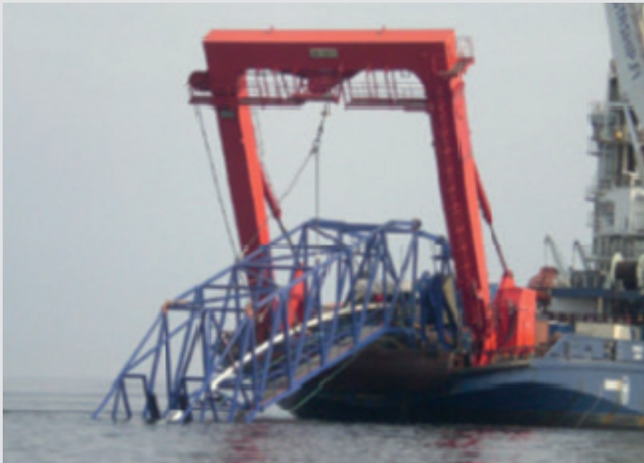
Figure 5: Stinger on Pipelay Vessel
